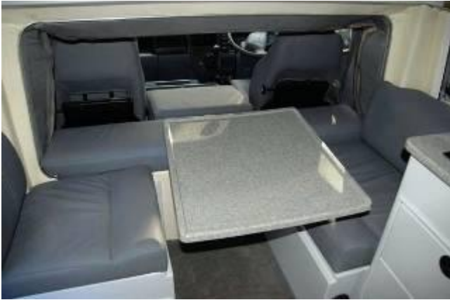
Up front are two leather seats, with a swing-away table. The table will in fact swing completely into the vehicle cab if needed, or drop down to form a single bed if required. To the right is the ceramic diesel cooktop and more storage.
