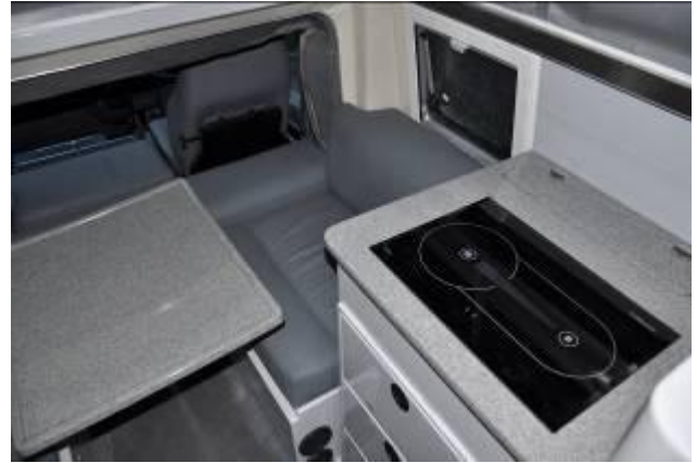
Up front are two leather seats, with a swing-away table. The table will in fact swing completely into the vehicle cab if needed, or drop down to form a single bed if required. To the right is the ceramic diesel cooktop and more storage.
